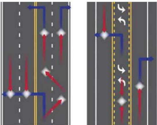
*Mid-Block Conflict Points for Four-Lane Undivided Roadway and Three-Lane Cross Section (Adapted from Welch, 1999)<sup>4</sup>*
